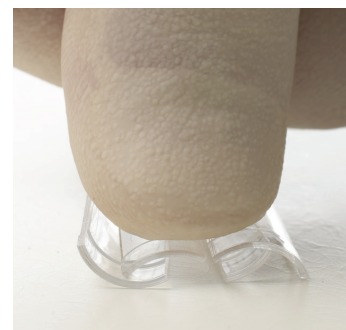
Other brands of culture tubes have thin walls that crush easily
