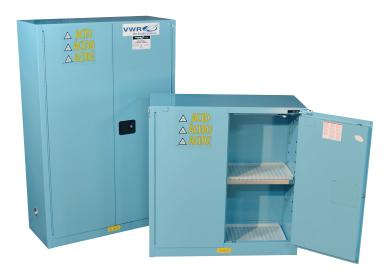
VWR Safety Cabinets are designed to protect both laboratory personnel and the cabinet contents. Fully welded, 18-gauge steel ensures fire protection and strength with reduced gaps. Equipped with upper and lower diametrically opposed side vents, a ground connector on lower right side of the cabinet, double-wall construction with 3.8cm (1½") insulating air space, and an environmentally friendly, electrostatically applied powder coat finish.
