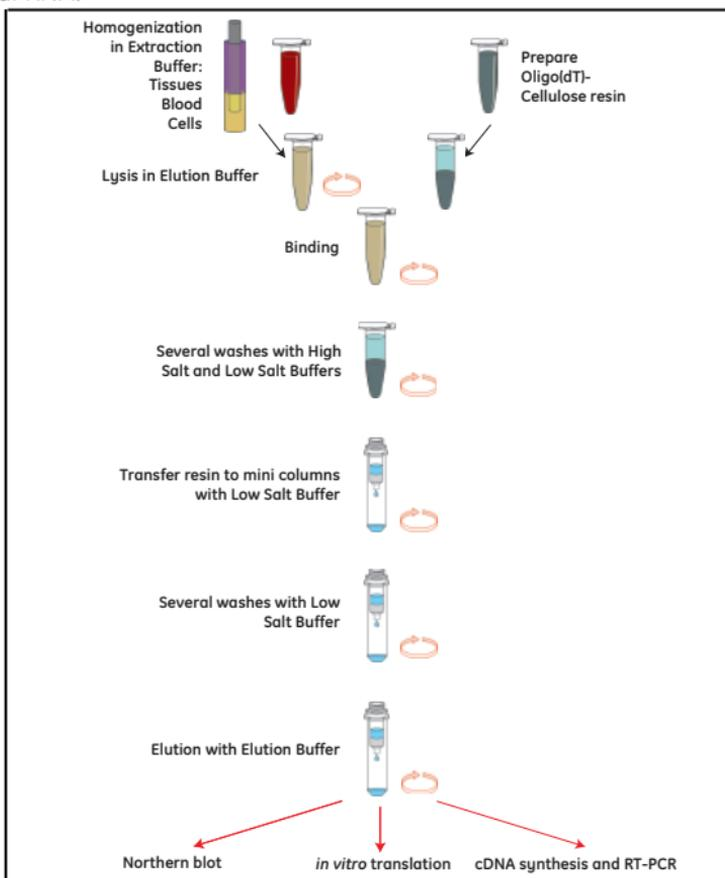
**Figure 4.1.** Overview of the **QuickPrep Micro mRNA Purification Kit** procedure
