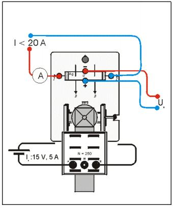
Fig. 3: Experimental setup (wiring diagram) for the Hall effect.
