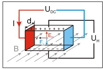
The Hall voltage  $U_{\text{H}}$  is caused by the deflection of the moving charge carriers in the magnetic field due to the Lorentz force, whose direction may predicted by the right hand rule. The
