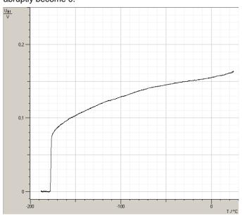
Fig. 4: Voltage drop at the transition temperature of approximately -180 °C.
