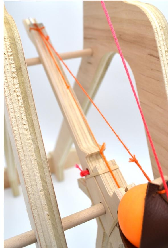
11) Check that the center of the swing arm is aligned with the center of the pulley. IF YOU DO NOT DO THIS THE TREBUCHET IS LIKELY TO MISFIRE.
