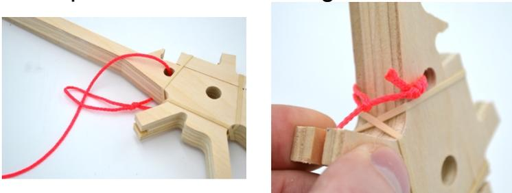
9) Attach the swing arm to the A-frame using the 8.5" long dowel. The swing arm should be oriented so the release pin is up when the throwing arm is pointing forward. The dowel is not intended to be glued to either the swing arm or the A-frame, but is allowed to rotate freely.
