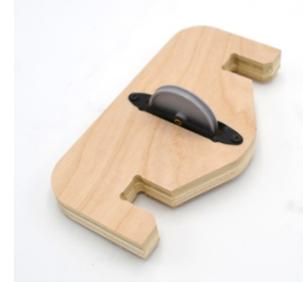
3) Insert the pulley mount into the forks for the pulley mount with the screws to the front of the trebuchet. The top of the pulley mount should be level with the top of the forks when seated properly.
