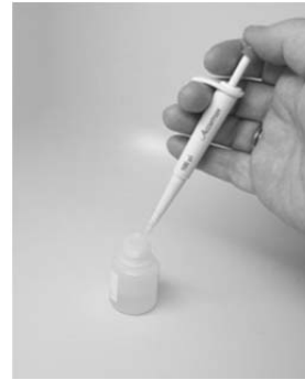
Withdrawing Standard Solution Using Pipette
