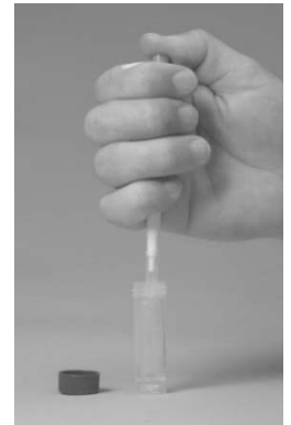
Transferring Spike Solution to Sample Tube
