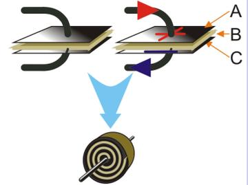
Normally, the metal sheets are uncharged. When an electric current flows, one plate becomes positively charged, and the other negatively charged. This storage of charge is how the capacitor stores energy.
