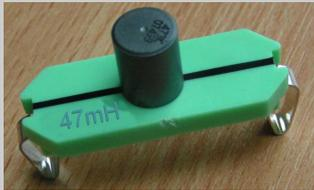
Resistors oppose electric currents. Inductors oppose *changes* to electric currents, but the mechanism is different.
