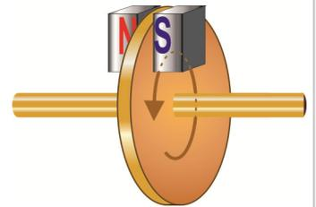
The braking effect is varied by adjusting the current to the electromagnet. As the spinning disc slows, the induced eddy currents decrease, reducing the braking effect. In this way, the vehicle is braked smoothly.
