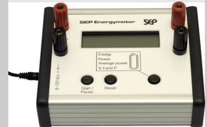
Here, it is used to measure the energy stored in a capacitor.
