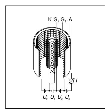
Fig. 1: Schematic diagram of the mercury Franck-Hertz tube
