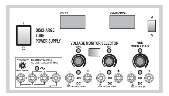
The power supply ESRDS1337 Discharge Tube Power Supply is a very useful & unique Power Supply which provides the High Voltage (10 to 500V & 0 to 80V) & Low Voltage (0 to 20V DC, 5 Amps.) along with the DIGITAL DISPLAY for Voltage & Current. It also provides the AC Voltage selectable from 1 to 6V AC, 2 Amps. All the outputs provided are independent of each other and can be used simultaneously.
